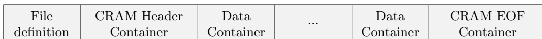
Figure 1: A CRAM file consists of a file definition, followed by a header container, then other containers.
