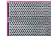
Microfluidic chip guides flow. Fabricated using mr-I T85. 200 nm deep holes, maximum hole size: 500 nm diameter (courtesy of HEC / TU Darmstadt)
