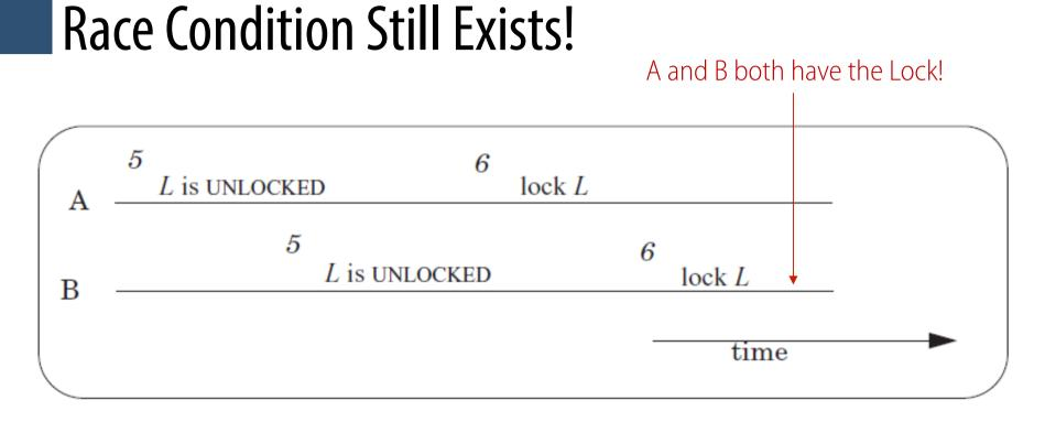
Operation-1: Read L to check if its state is LOCKED Operation-2: Write L to change its state to LOCKED
