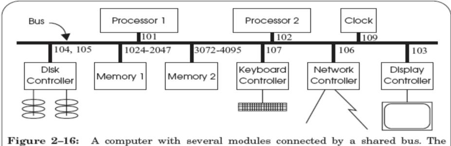
Figure 2–16: A computer with several modules connected by a shared bus. The numbers are the bus addresses to which the attached module responds.
