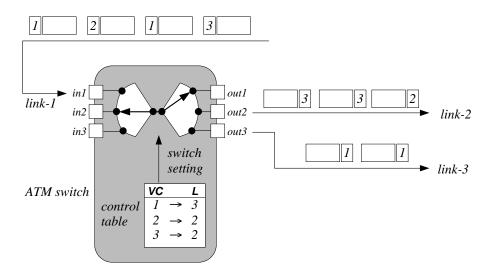
Figure 9.23 The principle of an ATM switch.
