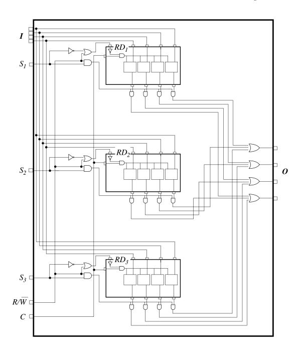
Figure 2.21 A naive construction of a three 4-bit word memory chip.
