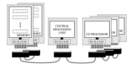
Figure 3.14 A general interconnection scheme by means of a single backplane bus.
