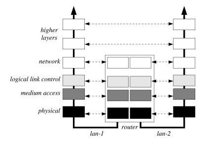
Figure 9.1 The position of a router in terms of the OSI reference model.
