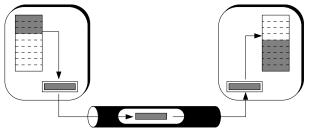
transmit frame # k+1 from sender to receiver
