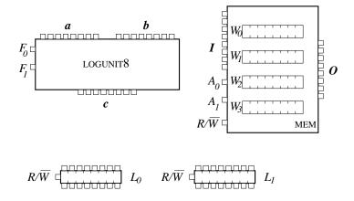
**Figure 3.1** The available components: the IC LOGUNIT8, a four 8-bit word memory MEM, and two 8-bit words  $L_0$  and  $L_1$ .
