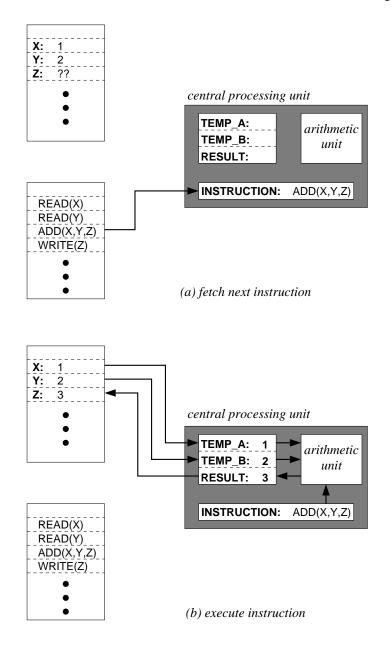
**Figure 1.6** The organization of a computer in which an instruction is fetched (a) and subsequently executed (b).
