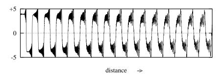
Figure 7.5 The effect of delay distortion when transmitting a digital signal.
