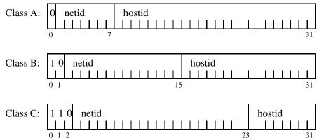
Figure 9.16 The address layout for the first three classes of the Internet addressing convention.
