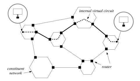
Figure 9.12 The construction of a virtual circuit in an internetwork.
