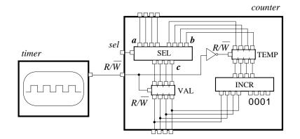
Figure 2.20 An implementation of a 4-bit counter.
