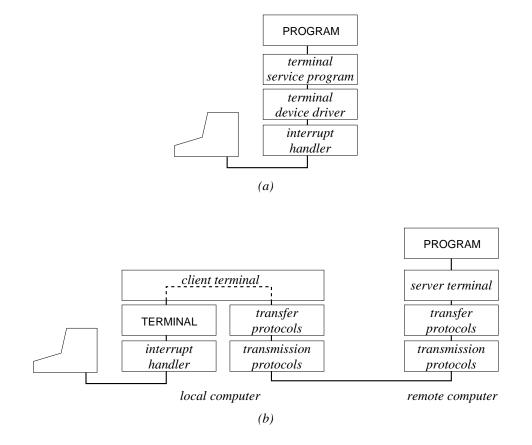
**Figure 10.6** The principal working of a virtual terminal (b). The original situation is shown in (a).
