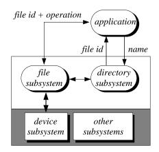
Figure 5.22 The organization of a file system and directory package on top of a microkernel.
