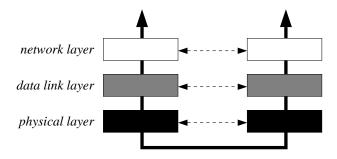
Figure 7.26 The three lower layers of the OSI reference model.
