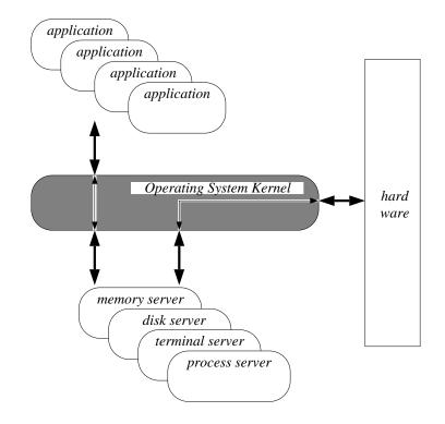
Figure 5.19 A client-server architecture applied to an operating system.
