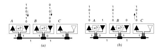
Figure 8.2 Detecting collisions by station *B* (a) and *A* (b).
