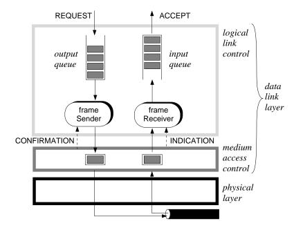
Figure 8.15 The outline of a software solution for queuing incoming and outgoing data.
