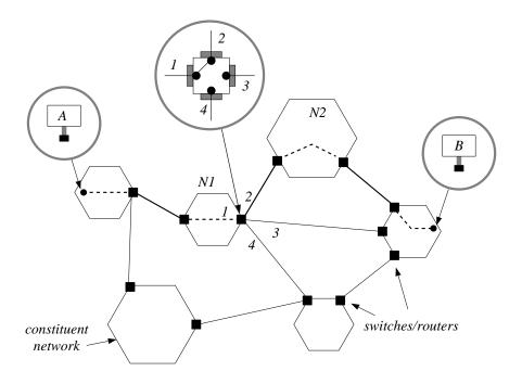
Figure 7.14 The principal working of a circuit-switched network.
