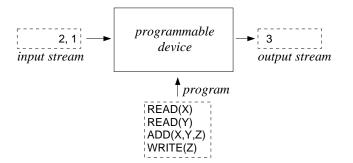
Figure 1.5 The principle of a programmable device.
