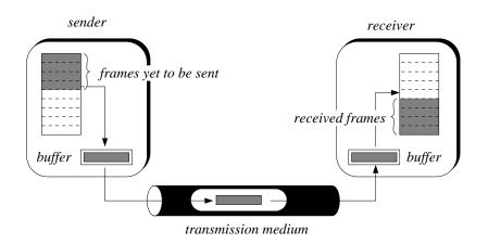
Figure 7.16 The principle of frame transmission.
