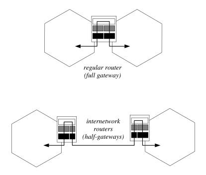
Figure 9.10 Using internetwork routers to construct an internetwork.
