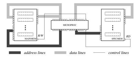
Figure 3.12 The implementation of a bus by direct wiring.
