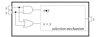
Figure 2.9 Outline of an implementation integrating two different operations.
