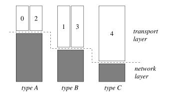
Figure 9.24 The relationship between transport protocols and different network types.
