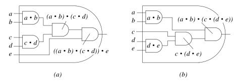
Figure 2.5 The construction of an AND gate with five input lines.
