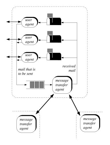
Figure 10.11 The general organization of a message handling system.
