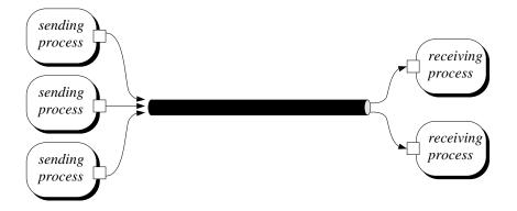
Figure 6.12 The principle of a channel in message-based communication.
