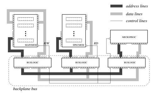
Figure 3.13 Connecting components by means of a backplane bus.
