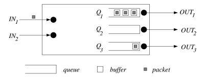
Figure 9.3 Accepting and storing incoming packets at a router.
