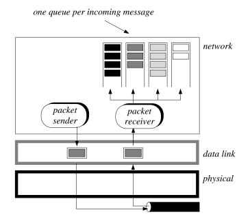
Figure 9.11 The principle of reassembling subnet packets to their original internet packet.
