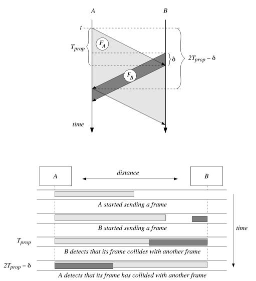
**Figure 8.4** The detection of collisions in CSMA/CD protocols requiring a contention period of  $2T_{\text{prop.}}$
