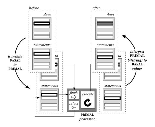
Figure 4.6 Simulating the BASAL fetch-execute cycle by the PRIMAL processor.
