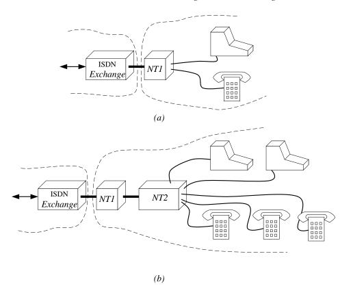
**Figure 9.20** The use of network terminating devices at a customer's premises for (a) basic services and (b) primary services.
