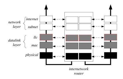
Figure 9.8 The subdivision of the network layer into two sublayers to support internetworking.
