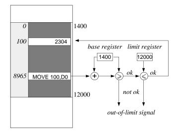
Figure 5.3 Using hardware to check if addresses are referenced within the proper limits.
