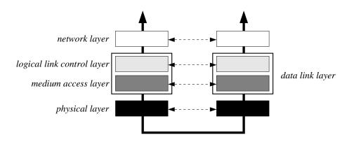
**Figure 8.3** The position of the medium access and the logical link control layer in the OSI model.
