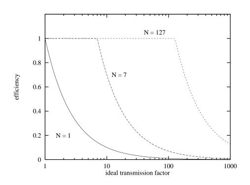
Figure 7.19 The efficiency of a transmission medium when using a sliding-window protocol.
