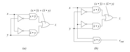
Figure 2.6 An implementation for the exclusive-or function (a) and a half adder (b).
