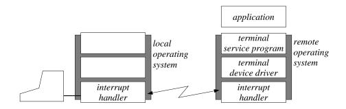
Figure 10.5 Having a remote device driver control a local terminal.
