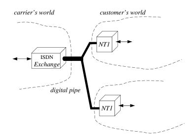
Figure 9.19 The basic architecture for an ISDN connection.
