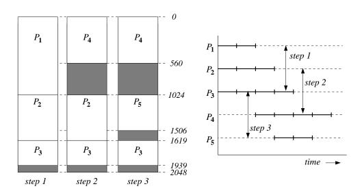
Figure 5.4 Placing programs into memory.
