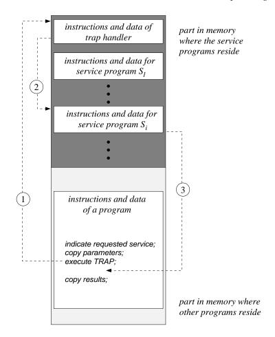
**Figure 5.12** The interaction between service programs and a program requesting a service *\$*to be performed.
