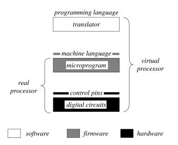
Figure 4.1 The relation between real and virtual processors.
