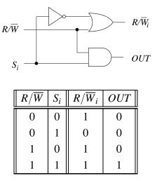
Figure 2.22 The basic digital circuit for selecting a word and its associated function table.
