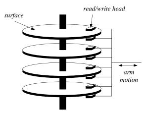
Figure 3.19 A typical organization of a hard disk.
