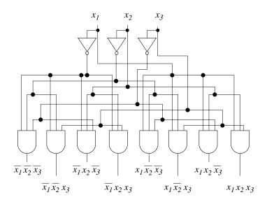
Figure 2.23 A 3-to-8 decoder circuit.
