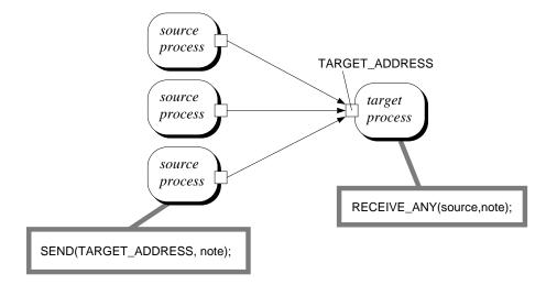
Figure 6.3 The situation of passing notes from several source processes to one target process.
