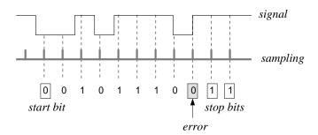
Figure 7.9 The effect of a receiver sampling too quickly for an incoming signal.
