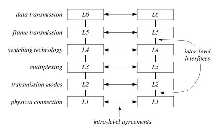
Figure 7.25 The principle of layered agreements.
