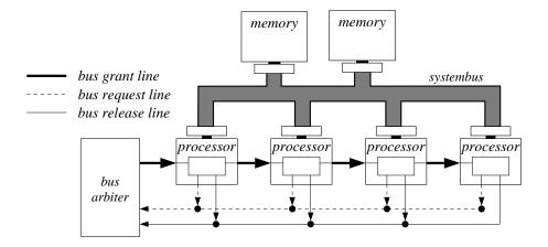
**Figure 3.15** Requesting bus transfers by several masters through centralized daisy chain arbitration.
