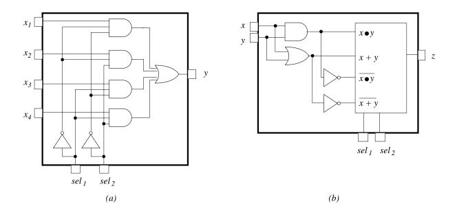
**Figure 2.11** An implementation of a selection mechanism for four inputs (a), and its application in an integrated circuit (b).
