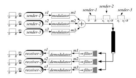
Figure 7.22 The principle of frequency-division multiplexing.
