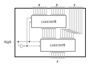
Figure 3.2 Cascading two circuits LOGUNIT8 in order to directly implement computation (3.1).
