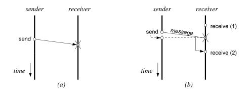
**Figure 6.8** Buffered communication using message-discarding (a) without and (b) with information on success of transmission.
