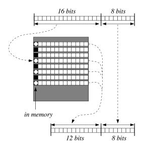
Figure 5.8 Address conversion in virtual memory systems.
