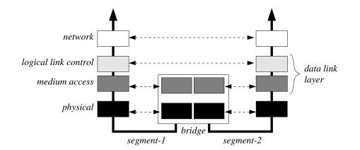
Figure 8.8 Connecting two LANs by means of a bridge.
