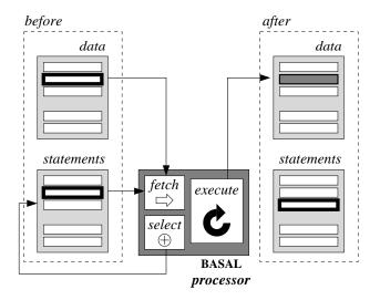
Figure 4.5 The effect of fetching and executing a BASAL statement.
