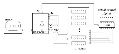
**Figure 3.6** The outline of a mechanism for controlling the automated execution of micro-instructions.
