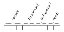
Consequently, in order to have the microroutine ADD01T03 executed, we need to provide the bit string  $\langle 001 \ 00 \ 01 \ 11 \rangle$ . This bit string then needs to be *interpreted* by the microcalculator as an ADD microroutine, operating on the contents of registers REG0 and REG1, and of which the result is to be stored in REG3. In other words, this instruction
