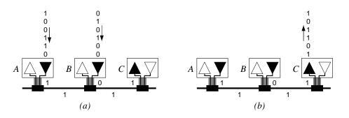
Figure 8.1 The effect of colliding messages, at the start (a) and end (b) of transmission.
