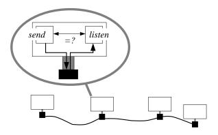
Figure 1.13 The principle of detecting message collisions.
