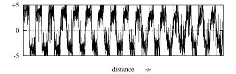
Figure 7.6 The possible final result of sending a digital signal across a line.
