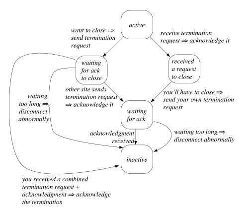
Figure 9.25 A state transition diagram for closing a connection. Adapted from Stallings(1994).
