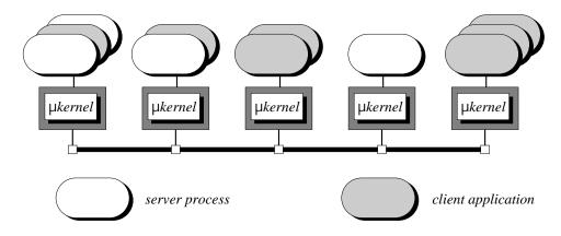
Figure 5.20 A distributed version of a client-server based operating system.
