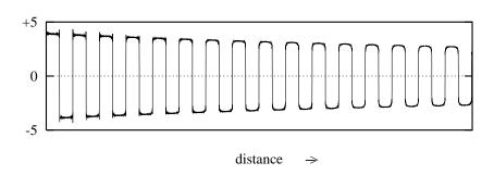
Figure 7.4 The effect of frequency-dependent attenuation on a digital signal.
