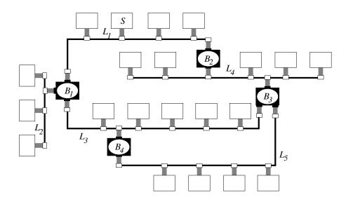
Figure 8.12 A network containing a cycle.
