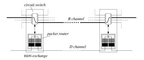
Figure 9.21 Establishing a circuit-switched based connection in an ISDN.
