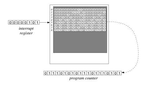
Figure 5.11 The principle of an interrupt table.
