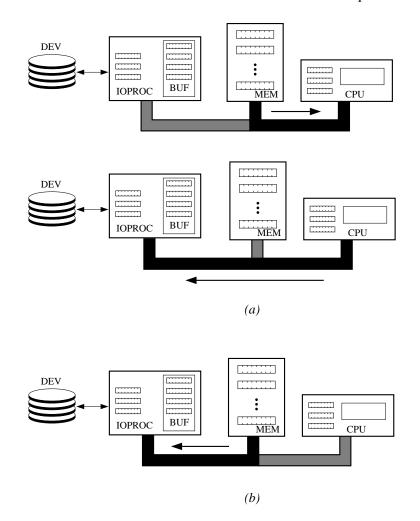
**Figure 3.17** Transferring data for output via the CPU (a), or by means of direct memory access (b).
