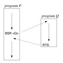
Figure 4.3 The principle of calling and executing a subroutine in PRIMAL.
