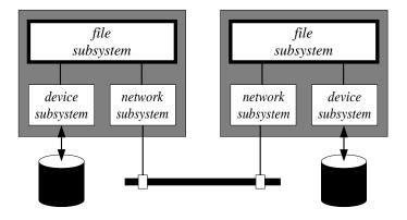
**Figure 5.13** The global interaction between two different operating systems connected in a computer network.
