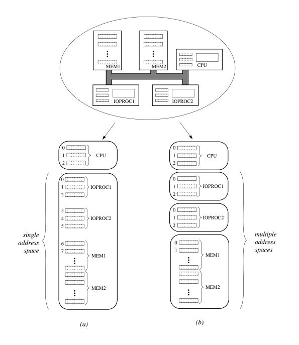
**Figure 3.16** Mapping memory and registers into a single address space (a), or into different address spaces (b).
