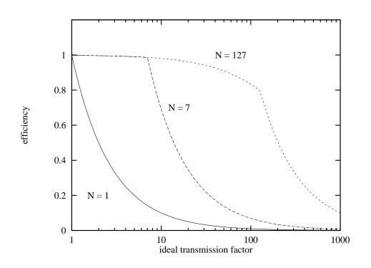
Figure 7.20 The efficiency of a transmission medium when using a sliding-window ARQ.
