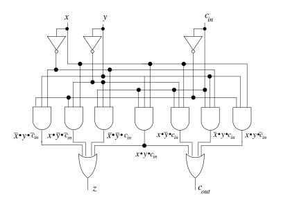
Figure 2.8 An implementation for the full adder operation.
