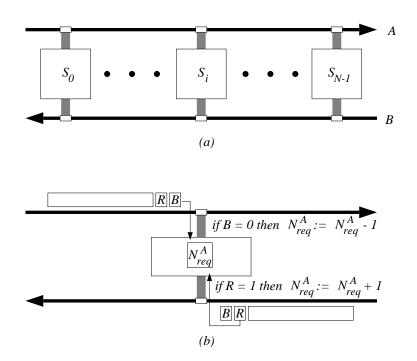
Figure 8.11 The architecture of a DQDB network (a) and its principal operation (b).
