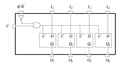
Figure 2.18 The layout of a 4-bit word integrated on a single chip.
