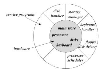
**Figure 1.8** An operating system viewed as a collection of service programs shielding the hardware.
