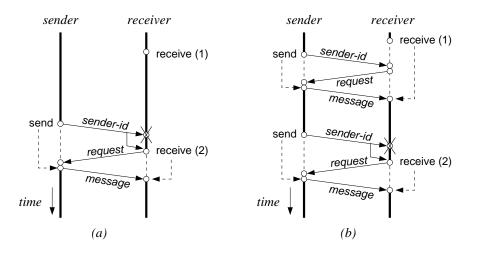
**Figure 6.11** The refinement of synchronous communication with finite input queues using (a) non-blocking receive, and (b) blocking receive.
