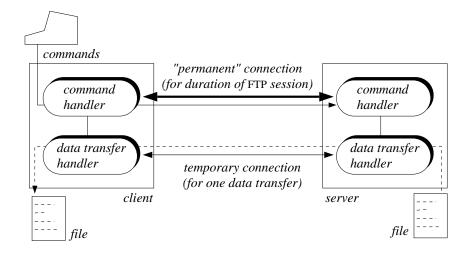
Figure 10.8 The architecture of Internet's FTP.
