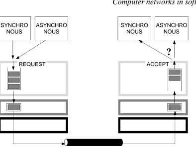
Figure 8.17 The organization of the two communication modules with respect to the OSI layers.
