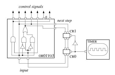
Figure 3.8 A hardwired control of three execution steps.
