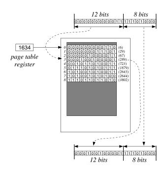
Figure 5.6 Address conversion in paged computer systems.
