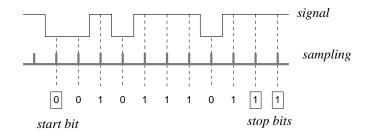
Figure 7.8 Bit synchronization by using start and stop bits.
