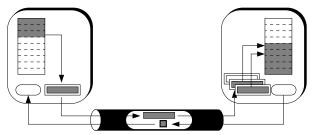
*transmit frame # k+1 from sender to receiver, and return an acknowledgment for frame #k*
