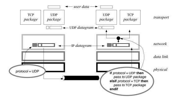
Figure 9.17 The transmission of a UDP datagram.
