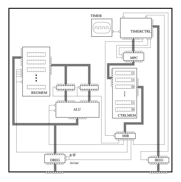
Figure 3.9 The architecture of a simplified microcalculator.
