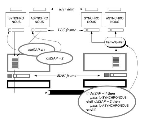
Figure 8.18 Handling incoming frames for different communication protocols.
