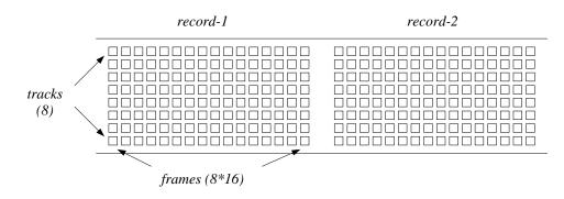
Figure 3.18 The organization of magnetic patterns on a tape.
