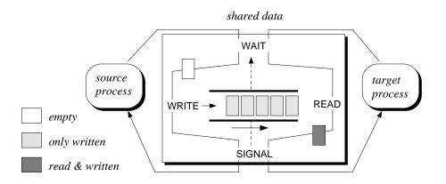
Figure 6.2 The principle of communicating by means of a shared stream.
