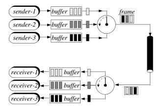
Figure 7.23 The principle of time-division multiplexing.
