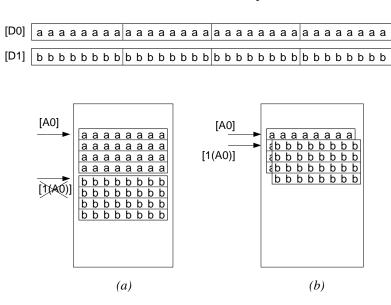
Figure 4.2 The effect of indexed addressing in PRIMAL.
