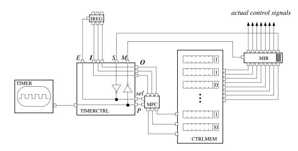
Figure 3.7 The actual control mechanism for the execution of microroutines.
