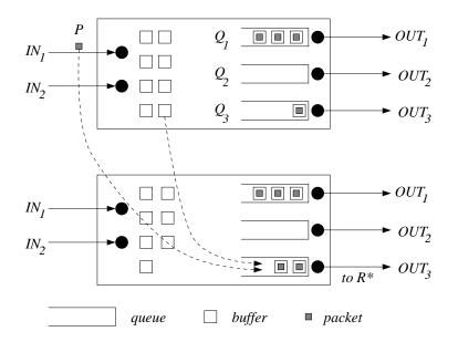
Figure 9.4 Allocating a buffer for an incoming packet destined for link OUT5.
