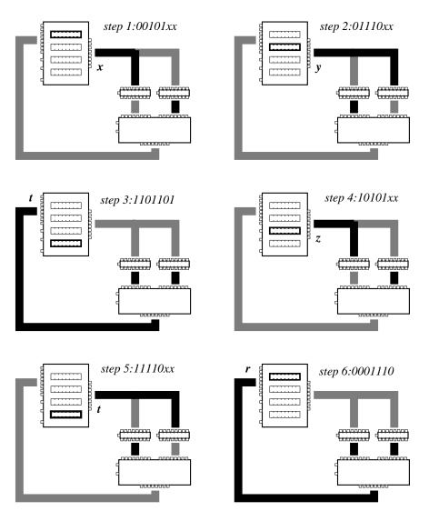
**Figure 3.4** Six sequentially executed steps for calculating  $(x + y) \cdot z$ .
