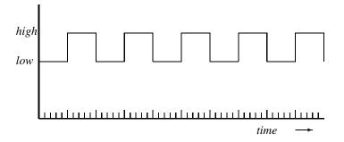
Figure 2.19 The signal produced by a timer.
