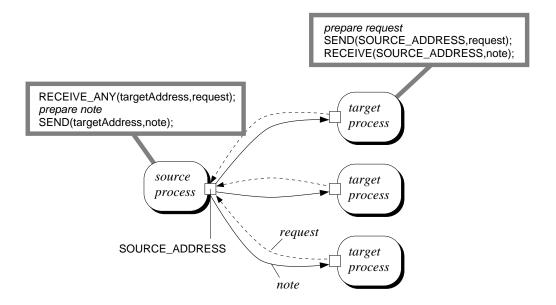
Figure 6.4 Passing notes from one source process to one of many target processes.
