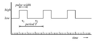
Figure 2.16 A characteristic clock signal.
