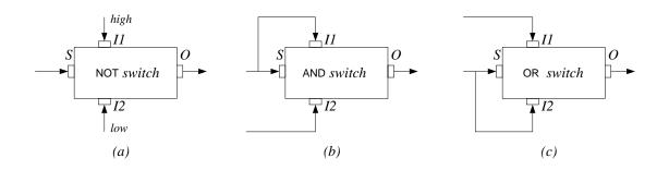
Figure 2.3 Wiring switches for construction of gates.
