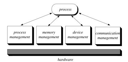
Figure 5.15 The overall architecture of a microkernel with four modules.
