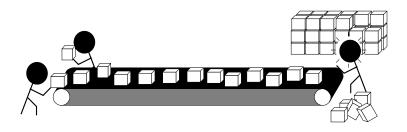
Figure 1.11 The effect of not properly balancing the work on a conveyor belt.
