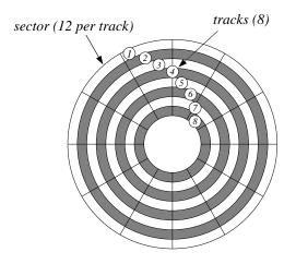
Figure 3.20 Layout of a surface of a hard disk.
