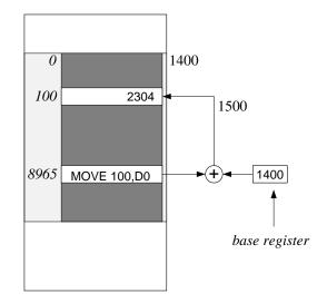
Figure 5.2 Using relative addressing and its conversion to absolute addresses.
