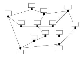
Figure 1.15 A computer network based on point-to-point links.
