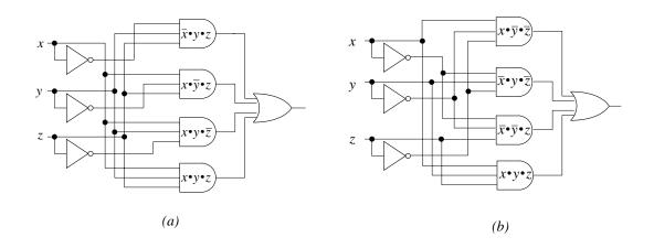
**Figure 2.7** An implementation for the majority function major3 (a), and the oddbits function odd3 (b).
