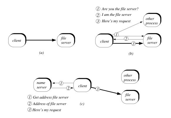
**Figure 10.14** Three ways of identifying processes: (a) using direct naming, (b) broadcasting a request for identification, and (c) using a name server.
