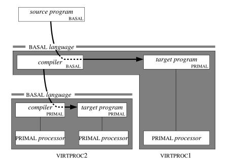
**Figure 4.9** The adapted architecture of the BASAL virtual processor, using a BASAL virtual processor (VIRTPROC2).
