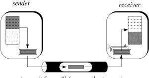
transmit frame #k from sender to receiver
