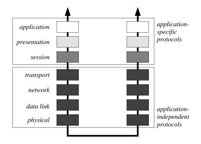
Figure 10.1 The complete OSI reference model.
