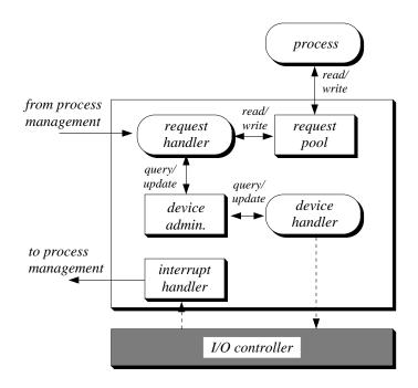
Figure 5.18 The general architecture of a device driver.
