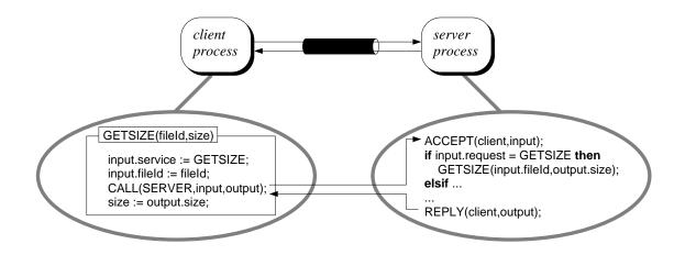
Figure 6.14 The principle of a remote procedure call mechanism.
