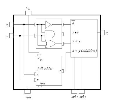
Figure 2.12 An implementation of a 1-bit ALU by integration of several circuits.
