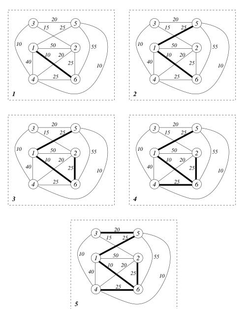
**Figure 9.6** An example of finding all least-cost paths originating at node 1, using Dijkstra's algorithm.
