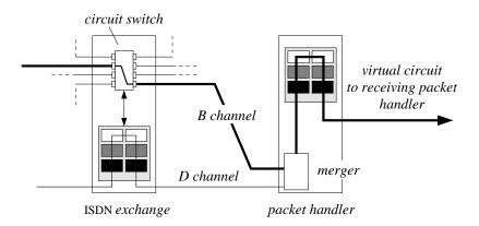
Figure 9.22 The principle of a packet-switched virtual circuit in ISDN.
