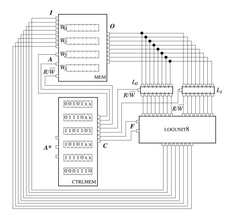
Figure 3.5 Adding a memory chip for storing settings of control lines.
