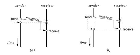
**Figure 6.10** Synchronizing two processes at the point of message receipt (a), and message delivery (b).
