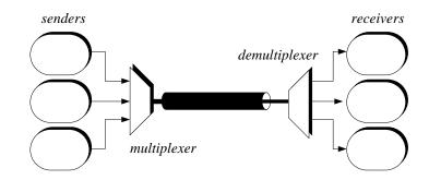
Figure 7.21 The principle of multiplexing a transmission medium
