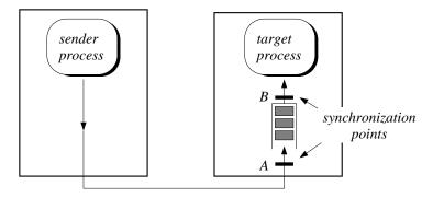
Figure 6.9 The two points of possible synchronization in message-based communication.
