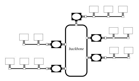
Figure 8.10 Using a backbone to connect multiple LAN segments.
