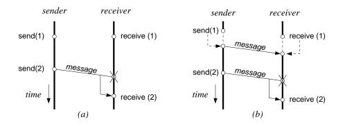
**Figure 6.7** The basic message-passing protocols for buffered communication using (a) nonblocking and (b) blocking communication.
