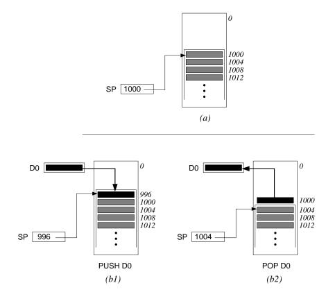
**Figure 4.4** The organization of stacks in PRIMAL. (a) The initial situation; the effect of pushing an item onto the stack is shown in (b1); that of popping an item in (b2).
