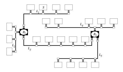
Figure 8.14 An example of five LANs connected by two bridges.
