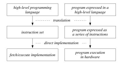
Figure 1.7 Viewing a computer as consisting of three distinct levels of instructions.
