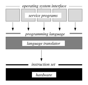
Figure 1.9 The construction of a virtual, multi-layered computing machine.
