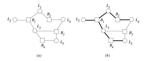
Figure 8.13 The representation of a network as a graph (a), and a tree spanning all its LANS (b).
