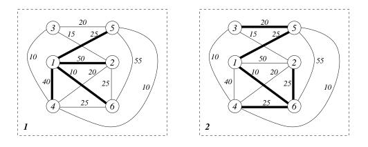
**Figure 9.7** An example of finding the least-cost paths originating at node 1, using the Bellman–Ford algorithm.
