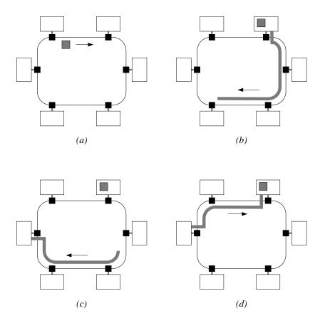
**Figure 8.5** The token ring mechanism: a token circulates (a), which is then claimed by a station that subsequently starts transmission (b). The frame arrives at its destination (c), and is later removed from the ring by its sender (d).
