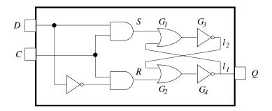
Figure 2.15 A clocked D-latch as a 1-bit memory.
