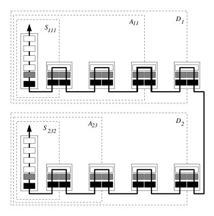
Figure 9.9 Passing a message across different networks through routers.
