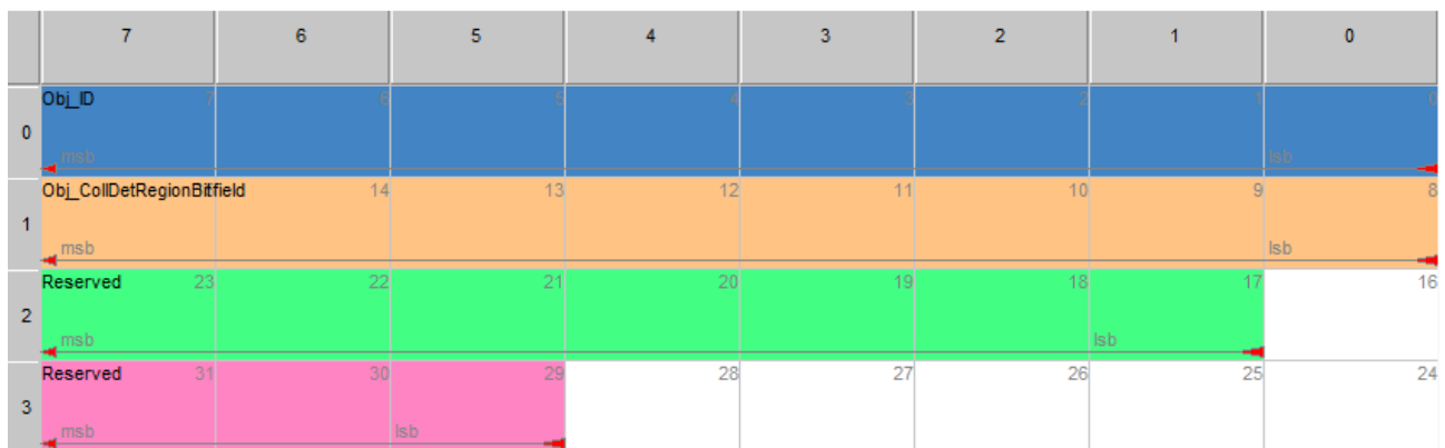
Figure 33: Object_4_Warning - message layout (0x60E)
