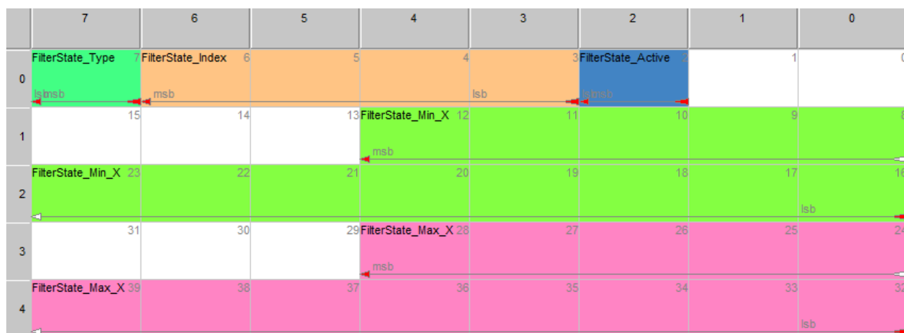
Figure 14: FilterState_Cfg - message layout for FilterState_Index=0xA (0x204) with 13 bit length for minimum and maximum value.
