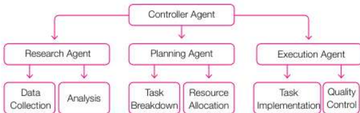
Fig 5.1: Hierarchical design with specialized agents performing specific tasks
