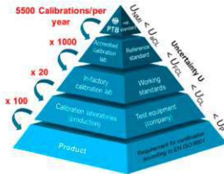
Figure 2. Representation of the calibration pyramid of the individual national metrology institutes/designated institutes and their integration in international interlaboratory comparisons with other NMIs/DIs.
