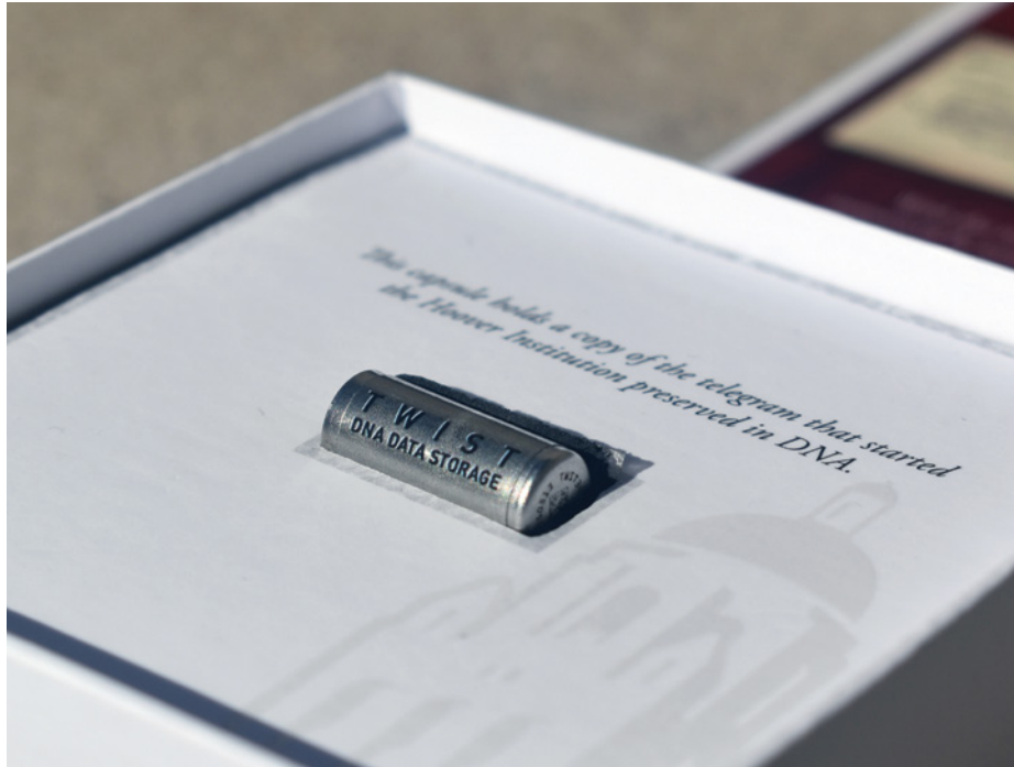
FIGURE 2.3 DNA is used as a storage medium for a digital copy of Herbert Hoover's telegram founding his namesake institution
