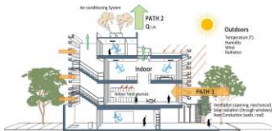
Fig. 5.1 The indoor-outdoor heat transfer and release, generating a negative loop of indoor overheating and outdoor extreme heat. (Source: Author)
