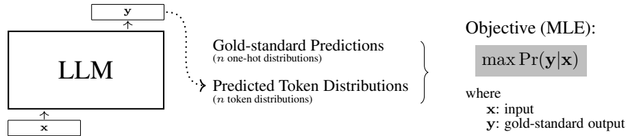
(a) Supervised fine-tuning (maximizing the prediction probability given the input)
