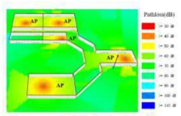
Figure 52: A sample scenario encompasses details of the floorplan and the path loss map computed with ray-tracer
