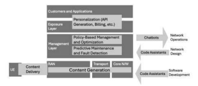
Figure 1: Overview of applications of LTMs in a mobile network.
