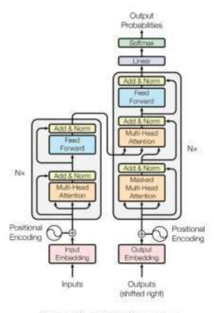
Figure 5: Transformers Architecture
