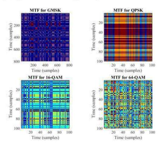
Figure 59: MTF Plots for various modulation schemes
