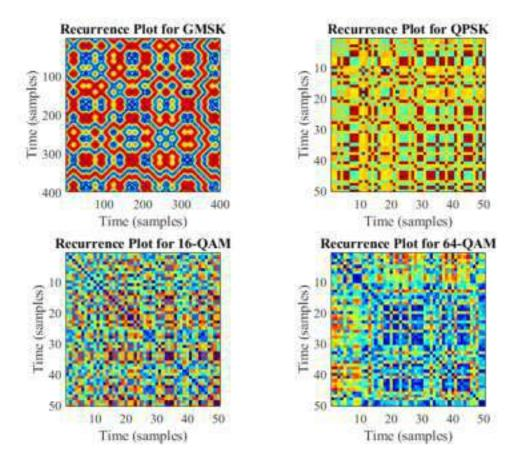
Figure 58: Recurrance Plots for various modulation schemes
