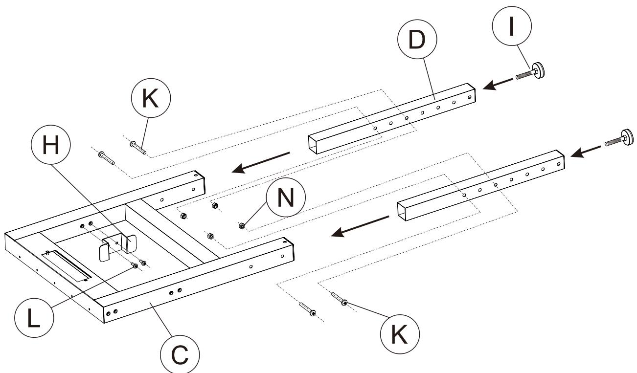
Install Adjustable leg,secure with bolts.
