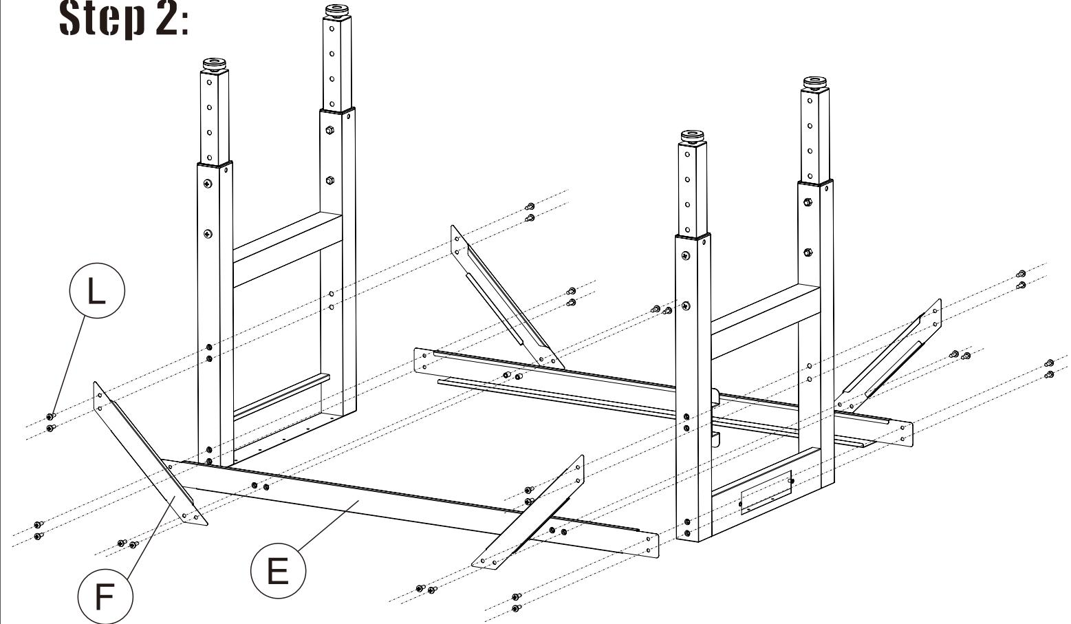
Secure the leg with B part and the side with F part.
