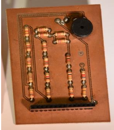
PCB with copper exposed, no solder mask or silkscreen.
