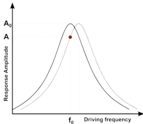
The response curve shows the amplitude of the cantilever (a driven oscillator) at frequencies near its natural frequency  $f_0$ .
