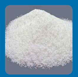
Borax decahydrate is a white colored inorganic powder having the formula  $\mathrm{Na_2B_4O_7}\cdot 10\mathrm{H_2O}$ . It occurs naturally as Evaporite, or as a combination of various hydrates of borax. Some of the major properties of borax are its high solubility in water, its ability to produce a yellowish green colored flame when ignited, it acts as a mildly alkaline salt, its good chemical stability, and it has good buffering and fluxing properties.
